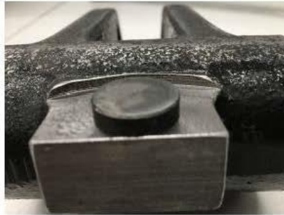
Figure 2: Brake Lever (AAA288AAG2) with Hardened Bearing Button
