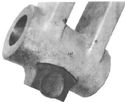
Figure 1: Brake Lever with Wear
